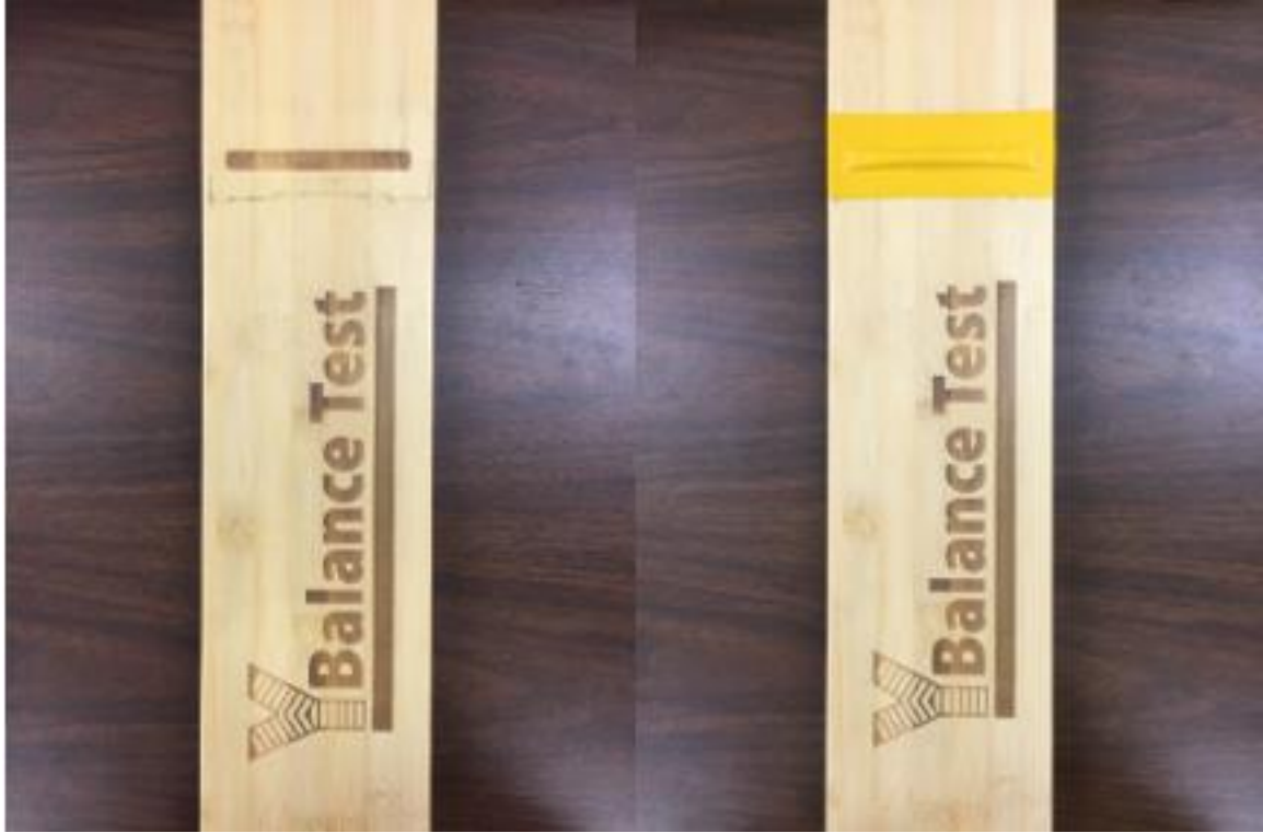
Figure 3.1 Side-by-side original (left) and modified (right) YBT stance platform. Note. On the modified stance platform, note the cylindrical shape (i.e., rolled tape) taped on top of the stance line used to provide tactile/haptic feedback.
